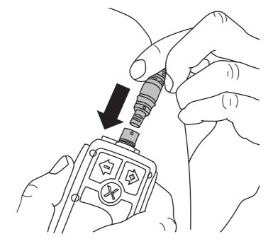
2. Connect a radio cable to the radio cable connector (6).
