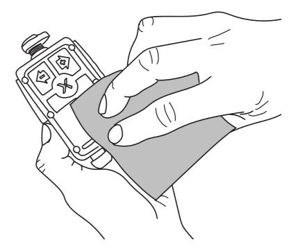
Clean the connectors and use Vaseline spray on the audio connector (female headset plug) twice a year (SAVOX recommends TURBO OIL PRF 290m manufactured by Taerosol, or similar type of lubricant).
